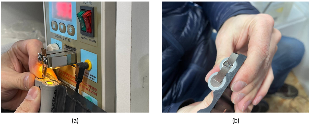
Figure 81: Battery soldering process: (a) Spot welding; (b) Magnesium strips
